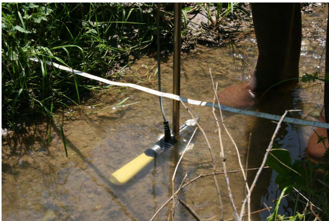
Picture 3. Measuring water flow using Ott Nautilus instrument on small experimental watershed Milanovac (Beomuzevic site)
